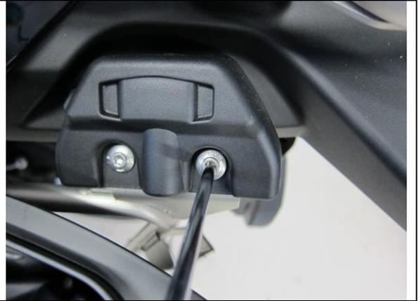
Assemble the M5 x 30 Torx bolt, thick M5 x 14 washer and aluminum spacer as shown at right. Install this into the bolt hole – secure lightly.
