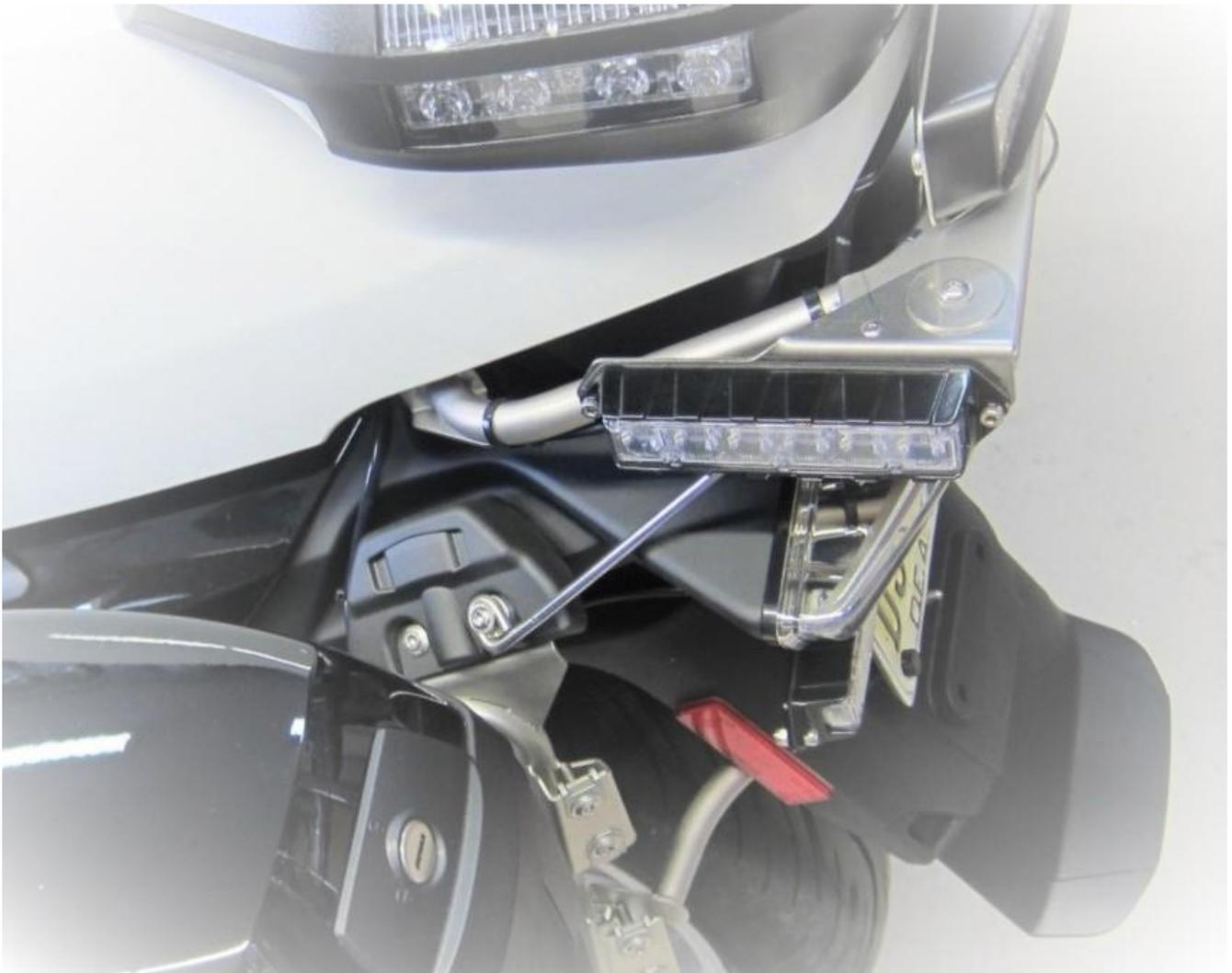
Remove the rearward bolt securing the saddlebag mounting bracket plastic covers. The hardware kit is shown below.
