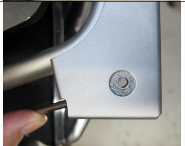
If you are installing a boomerang low band antenna mount, the additional body washer is not needed on the top side of the mount.
