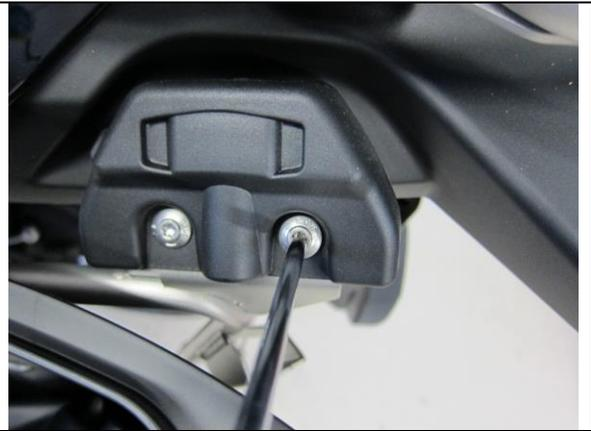
Assemble the M5 x 30 Torx bolt, thick M5 x 14 washer and aluminum spacer as shown at right. Install this into the bolt hole – secure lightly.
