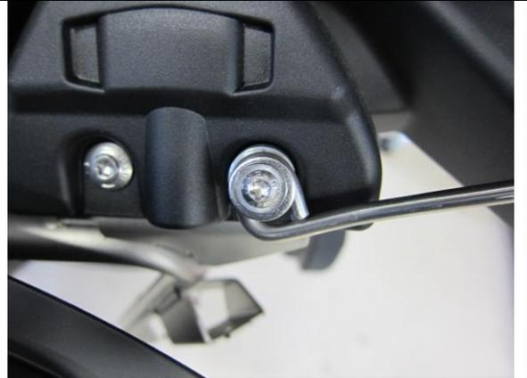
Position the other end of the strut so that it is in the center of the hole on the antenna mounting plate. Tighten securely the M5 x 30 Torx bolt from above.
